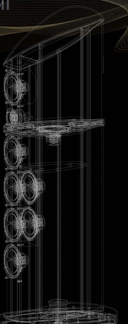
The Isobaric concept has been a central component in this pursuit of the ultimate low frequency performance. The smallest possible enclosure offers the lowest possible noise in conjunction with a controlled bass reproduction that is simply beyond the limitations of conventional, large diaphragm, slow woofer based designs.
